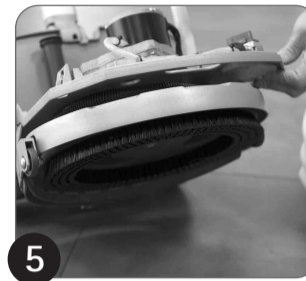
5 Check the wearing of the brush or pad holder ( do it without tanks )
