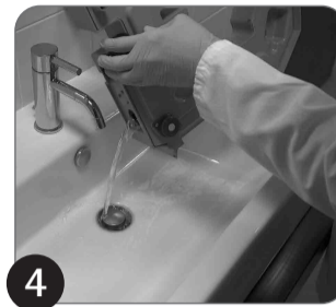
4 Empty the clean water tank
