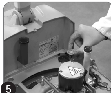
5 Clean the clean water filter
