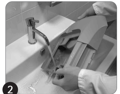
2 Clean the dirty water tank
