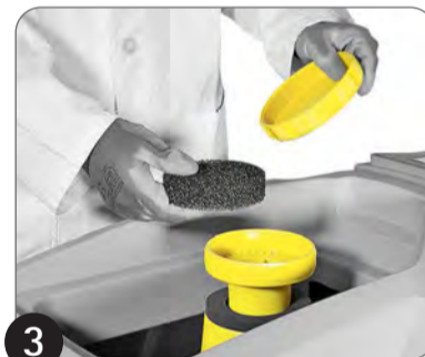
3 Check the condition of the float and the vacuum filter
