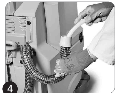
4 Clean the vacuum duct
